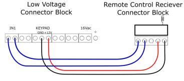
Mount the receiver on the right hand side of the Z-Series energiser. Connect +12V and 0V (GND) from the KEYPAD terminals on the energiser to the right-most terminals of the receiver, as per the diagram above.
